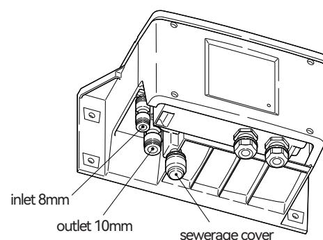
Note: Always tighten the fixing screws on the housing cover. If the screws are loose, the turbidity may not be measured correctly due to light entering the measuring tank or dust in the measuring water.
