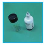
Take out the hardness test box, there are hardness indicator and sampling bottle inside
