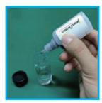
Drop the hardness indicator into the water sample and shake it continuously.
