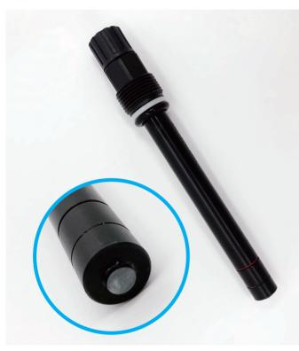
Note: If the electrode has been out of the water for approximately 30 minutes, then it is recommended that the electrode be put back into the water to regenerate for 1 hour.
